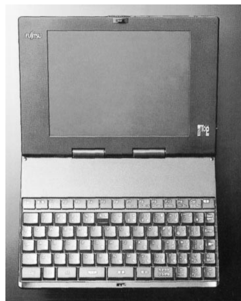
Figure 9. 7.2-inch color VGA screen and 15-millimeter key pitch keyboard.
