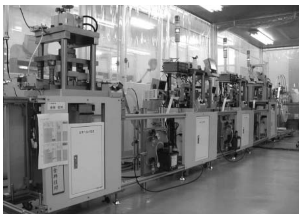
Figure 8 Mass-production line for automobile fuel injection nozzle plate.
